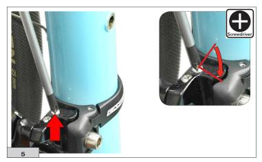
**6)** Tension the front derailleur cable firmly, and carry out an initial tightening (Fig.6).
