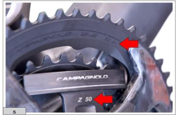
**3)** Fit the tool on the larger chainring having the hand crank almost in horizontal position, so that the longest teeth rest on the bottom of the tool's spline (Fig. 6).
