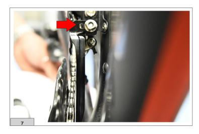
9) Adjust the CSD , leaving 1 mm of space between the chain (positioned on the smallest sprocket) and the CSD itself (Fig. 8).
